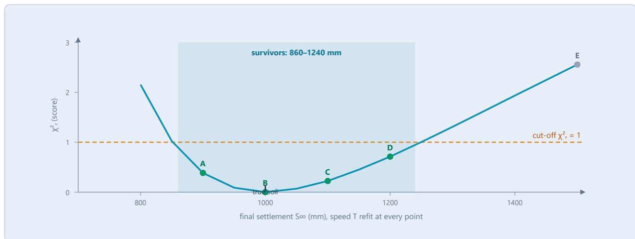
Figure 21.11. The score valley of the toy problem: for each candidate S_\infty the speed is refit and the best score plotted; the floor ( \chi^2_r \leq 1 , dashed) is nearly flat from 860 to 1240 mm. The toy uses a hard cut; the app uses score-weighting plus the fixed 95 % rule (§25.6). (Toy model; recomputable by hand.)
