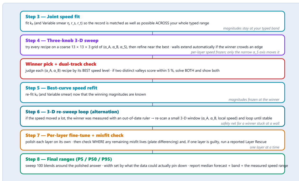
Figure 24.1. The Sweep Search pipeline and its rhythm: fit speed (teal) → sweep magnitudes (purple) → refit and re-check (teal) → polish and diagnose (amber) → report with uncertainty (green). Steps 1–2 set up the band; Step 6 loops back on itself.
