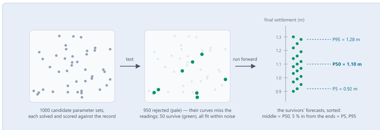
Figure 21.7. The 1000-candidate example: score all (left), reject the clear misses (middle — survivors green), sort the survivors' forecasts and read P5 / P50 / P95 off the column (right). (Schematic; dot counts reduced.)
