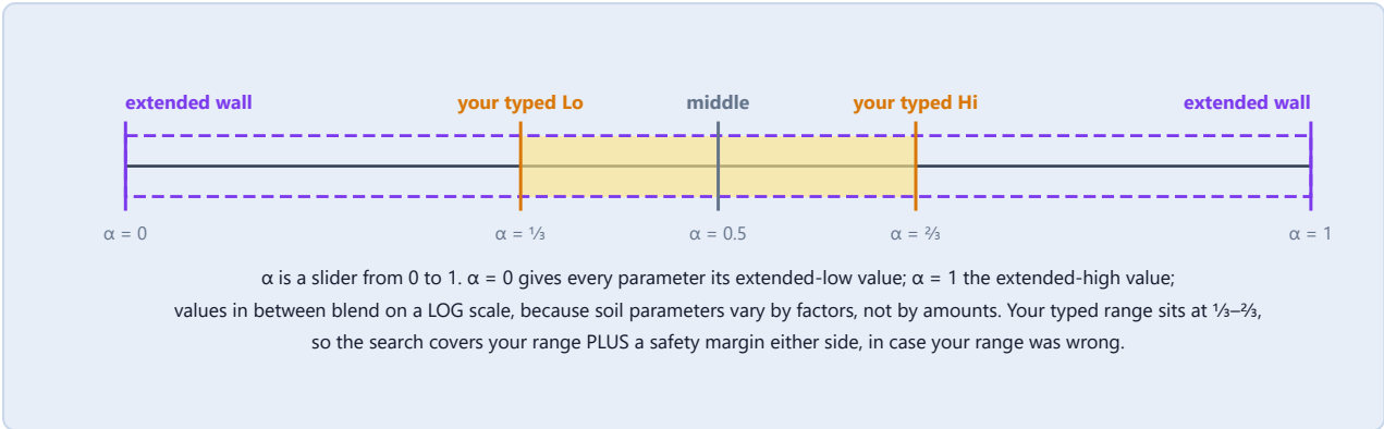
Figure 23.2. The \alpha ruler: each typed Lo–Hi is stretched threefold in log-width ( \text{exLo} = \text{lo}^2/\text{hi} , \text{exHi} = \text{hi}^2/\text{lo} ), so the typed values land at \alpha = \frac{1}{3} and \frac{2}{3} — the sweep checks your range plus a symmetric margin beyond it.
